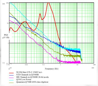
The Q330HR sets a new standard, requiring 26-bit resolution to fully represent its dynamic range. The 'HR exceeds GSN-class standard set by Quanterra nearly 20 years ago. The figure above shows the performance of the HR and standard channels in the Q330HR compared with the ultra-low-power Q330 and Quanterra's GSN-class Q730B. Better by a bit and at very low power!
