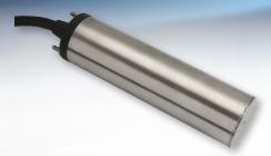
Model SBEPI is a *cost effective* triaxial downhole package useful for relatively shallow borehole installations. The unit consists of three EpiSensor force balance accelerometer modules mounted orthogonally in one small convenient package. The diameter of the SBEPI is only 2.625", making it suitable for installation in a 3" diameter hole.
